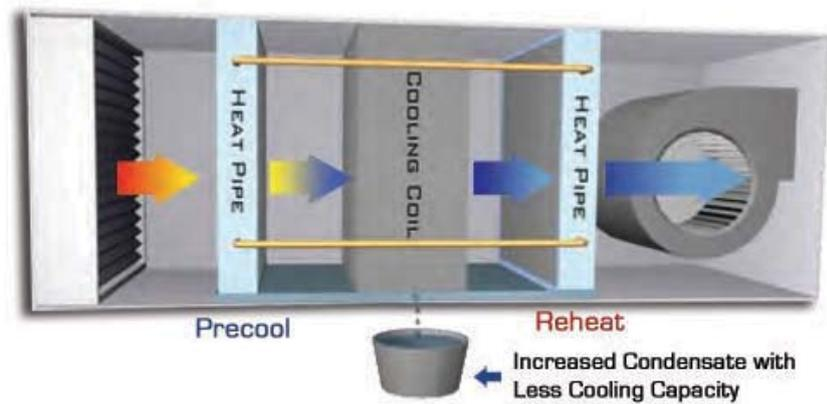
As hot incoming air passes over the precool coil, the liquid refrigerant vaporizes, absorbing heat from the air stream, thus lowering its temperature. This allows the cooling coil to run at a lower temperature. As a result more condensate is removed. Vaporized refrigerant then moves through connecting tubes to the reheat section downstream of the cooling coil, where it condenses, warming up leaving air and reducing its relative humidity.
